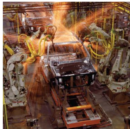
Figure 2: Spot-welding performed by robots on an assembly line
