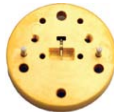
Monolithic InP-HBV chip mounted in a waveguide block
