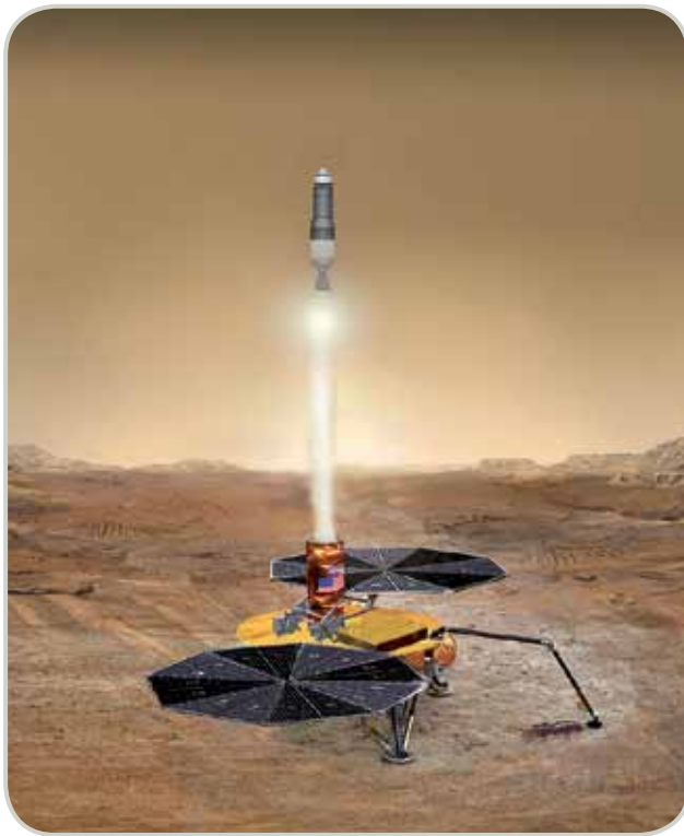
Solid propellant is considered for the Mars ascend vehicle. © NASA/JPL
